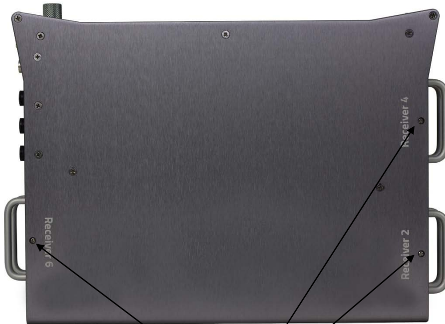
QRX212 Modules slide into the RX-12 with the arrow pointing to the top of the RX-12
