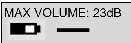
This menu allows you to set the maximum headphone output volume of the ERX. This can be useful if you are using the ERX mounted on a camera to feed audio and you want to set a level that will not be accidentally changed. If you set the volume mode menu to "fixed" the ERX audio will be the level set in this menu and will not be affected by the headphone knob.
