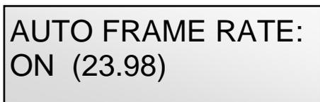
Auto frame rate sets if the ERX will automatically adjust its time code frame rate to match the incoming frame rate of the transmitter feeding it.
