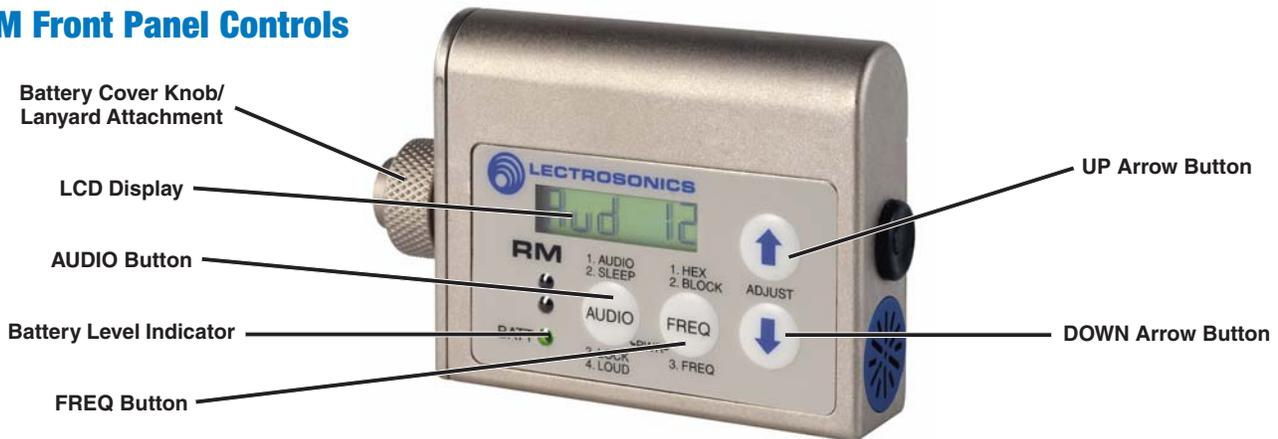
The RM unit gives you remote control of SM Series Transmitters using an audible tone delivered to the microphone in the wireless system. Operating parameters on the wireless transmitter can be set by holding the speaker on the RM close to the microphone and pressing the pushbutton. A “dweedle” tone will play from the RM speaker into the microphone and the parameter on the transmitter will be set immediately. Adjustments can be made to set:
