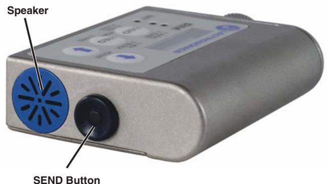
*The selected RM setting is relayed through a microphone attached to an SM transmitter via the RM speaker, and is activated by the SEND button above the speaker.*
