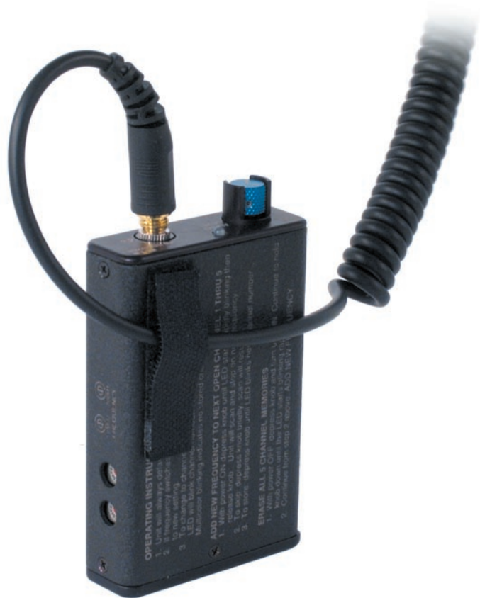
Figure 2 - Headphone cord strain relief
